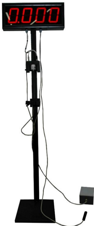
Figure 1.3: Free fall and Atwood machine experiment set-up.
